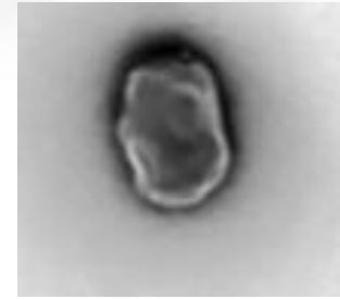
Pad or brush debris EDX = C, N, O → polyurethane pad EDX C, O only → brush
